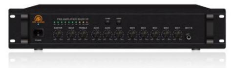
In the pa system the <u>Preamp RH2011P</u> takes whatever source it gets from microphone,CD/USB player or FM/AM tuner, and prepares that signal with a medium to high output impedance and current for the power amplifier to drive loudspeakers.
