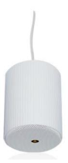
The RH-AUDIO Pendant Speaker RH-SL01 is designed for use where traditional ceiling mounted speakers are difficult or impractical to install, providing coverage angles of 360 degrees horizontal and 140~160 degrees vertical, giving an even dispersion over the audio spectrum.
