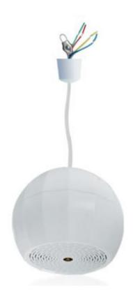
The <u>RH-AUDIO</u> Hanging Spherical Speaker RH-SL18 is built within an ABS resin bass-reflex enclosure using 5" cone-type pendant speaker driver and is intended for ceiling suspension installation, a 2 meter cable kit is included with a metal hook at the end.
