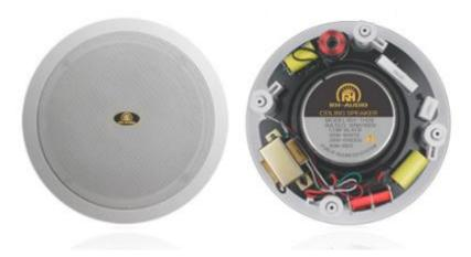
The <u>RH-AUDIO</u> In-Ceiling RH-TH26 is designed with professional two-way optimized crossover of unique round shape. The 6"long-throw polypropylene cone woofer with rubber surround is utilized for powerful middle and low frequency sound reproduction, while the 1"coaxially mounted silk dome tweeter round out the high sound pressure level.
